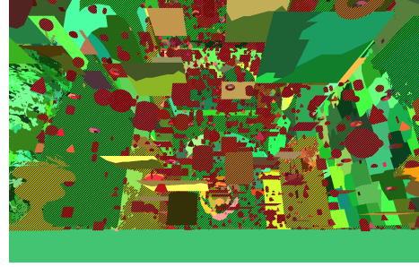
Figure 15: Debug visualization demonstrating per-mesh pipeline and LOD flexibility. Smooth surfaces with varied colors represent the Mesh Shader pipeline with meshlet visualization, while hatched surfaces indicate the Traditional Vertex Shader pipeline. The underlying color spectrum (green, yellow, orange, red) denotes varying LOD levels (0-3), highlighting that different meshes within the same model can utilize distinct pipelines, material types, and LODs simultaneously.
