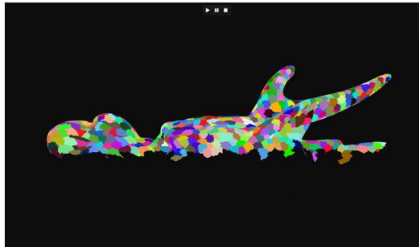
The Task Shader: Culls Invisible Meshlets
